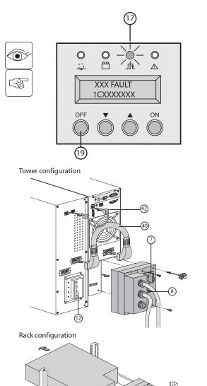
1. Stop the UPS with the OFF button (19) (press more than 3 seconds).
